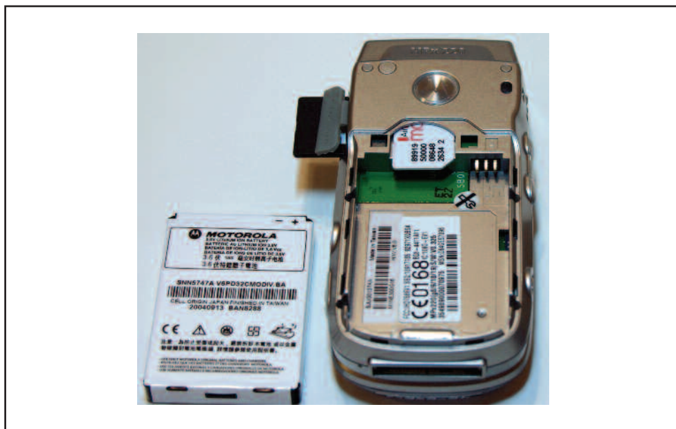
Figure 2 – Identification numbers potentially available from one handset
