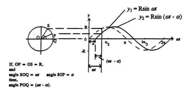
On the diagram, the curve for the phasor OS is  $y_1$  and that for the phasor OP is  $y_2$ . We can see from the circle on the left that,
