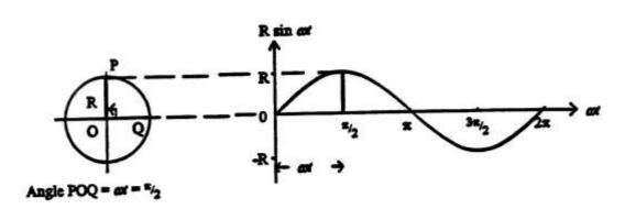
One complete cycle is completed whilst the radius OP turns through 360° or  $2\pi$  radians.
