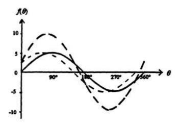
The values to be plotted for the resultant curve can be found by adding the height of the curve  $5\sin(\theta + 30^\circ)$  to that of  $5\sin\theta$  for each value of  $\theta$ .
