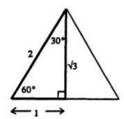
The equilateral triangle has been divided into two equal parts and the perpendicular height has been found by using the theorem of Pythagoras.
